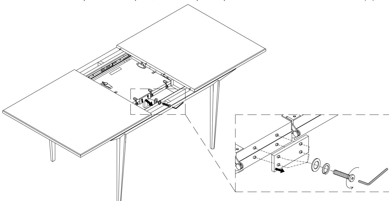
5. Lift the panel to unfold the middle leaf. Press the table ends back together. Tighten the table locks on the bottom side.
