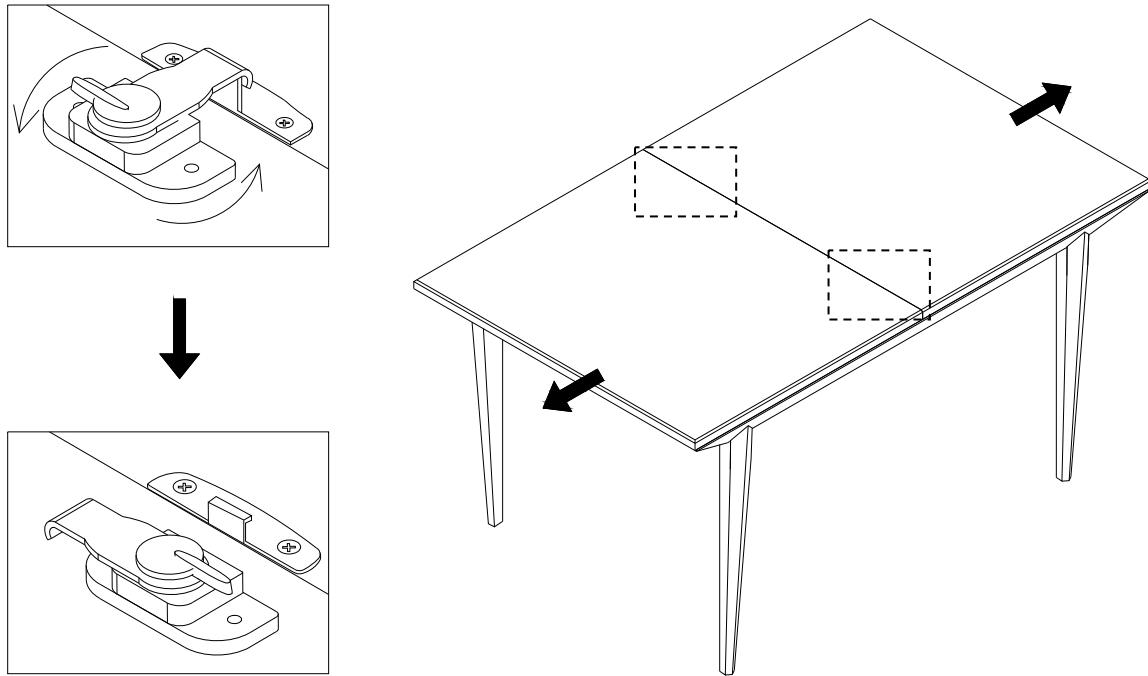
4. The block with the note label should be removed, unscrew the bolts as shown by using 4mm Allen Wrench (H).
