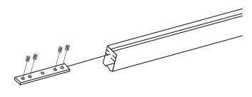
For connecting multiple tracks insert connector plate into middle level of track leaving approx 1 3/8" sticking out. Tighten 2 set screws with allen key into track so connector does not move.
