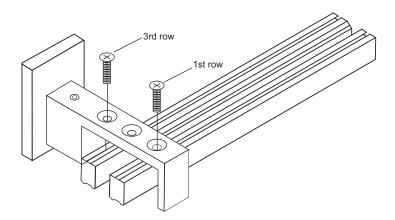
For single panel connect the track to the front row of screw holes in wall bracket.
