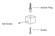
\*Mark desired distance between ceiling brackets on ceiling or inside of window. Each track requires two brackets.
