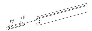
Insert connector plate into middle level of track leaving approx 1 3/8" sticking out. Tighten 2 set screws into track so connector does not move.
