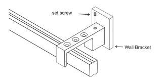
Place wall bracket over the loader and slide the bracket into position. Tighten the set screw with allen key.
