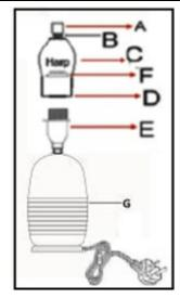
Unscrew shade ring (F) from the lamp holder & place harp metal ring (D) over the holder. Tighten with help of shade ring (F).
