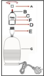
Unscrew the Finial (A) anti clockwise direction from the Harp Top (B).
