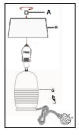
Place SHADE (H) (included) over the assembled harp, making sure the Harp Top (B) extends through the hole at the top of the Shade (H) (included). Attach the Finial (A) and tighten clockwise direction to secure the SHADE (H) (included).
