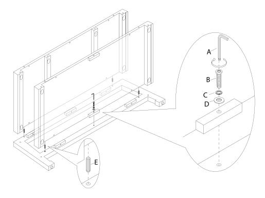
2. Fasten top and bottom panels to side panel using flat washer (D), lock washer (C), and screw (B) in order as shown. Tighten screws using allen key (A).
