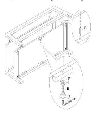
4. Fasten top and bottom panels to the side panel using flat washer (D), lock washer (C), and screw (B) in order as shown. Tighten screws using allen key (A).
