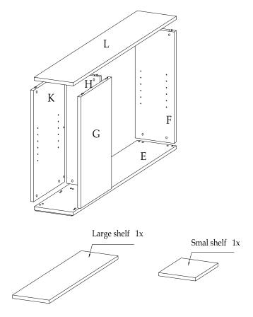
1. Put cam bolts (A) into pre-installed inserts on top panel (L) and bottom panel (E) as shown below. Tighten all cam bolts (A) with phillips head screw driver.
