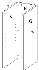
3. Carefully lift pre-assembled panels (K,G,H) onto bottom panel (E) by aligning cam bolts (A) with pre-drilled holes in panel (K), (G), and (H). Put cam houses (B) into pre-drilled holes in panel (K), (G), and (H) as shown below. Tighten all cam houses (B) with allen key (D).
