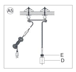
5. Unscrew the Knurled Nut (E) on the Socket (D).
