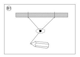
If needed, use a "stud finder" (not included) to locate the ceiling wooden joists and mark their locations on the ceiling using a pencil or a piece of tape. Mark the 2 slot locations of Screw Hooks (A) on ceiling joists at the desired locations
