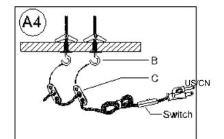
Position the Plastic Clips (C) along the cord so that they align with the installed Toggle Hooks (B) on the ceiling and carefully fit each Plastic Clip (C) onto each Toggle Hooks (B).
