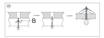
3. Use the Toggle Hooks (B), inserted through each of the 2 ceiling holes, making sure only the Toggle Hooks (B) are fully inserted into the ceiling and toggle wings are open. Rotate each Toggle Hook (B) clockwise until each flat washer on the Toggle Hook (B) is tight against the ceiling.
