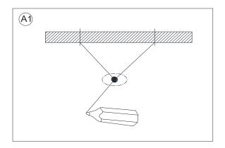
1. Mark the 2 slot locations of Toggle Hooks (B) on ceiling at the desired locations.
