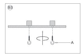
3. Insert Screw Hooks (A) into ceiling joist at the marked locations. Rotate each clockwise while firmly pressing it into the ceiling. Tighten Screw Hooks (A) securely into wood. If installing through drywall to wood joist, the threaded portion of each Screw Hook (A) will drive itself into the drywall and then into the underlying wooden ceiling joist.
