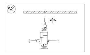
2. Using the drill with the appropriate size drill bit (just large enough to make hole that will allow passage of the folded Toggle Hooks (B), drill 1 hole in the ceiling at each of the 2 marked slot locations for the Toggle Hooks (B) assemblies.
