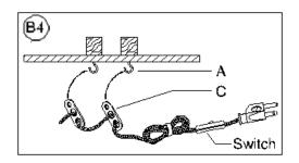
4. Position the Plastic Clips (C) along the cord so that they align with the installed Screw Hooks (A) on the ceiling and carefully fit each Plastic Clip (C) onto each Screw Hooks (A).
