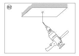
2. Pre-drill pilot holes at the marked locations. This will make installing the Screw Hooks (A) onto the wall easier.
