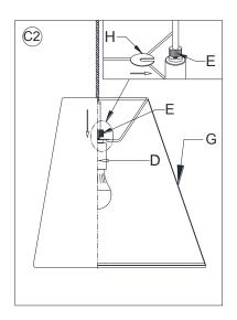
Position the Shade (G) over the Socket (D) by sliding the Horseshoe Ring (H) of Shade (G) onto the top of the Socket (D) as diagram, Secure the shade (G) to the Socket (D) by turning the Knurled Nut (E) by clockwise until tight.
