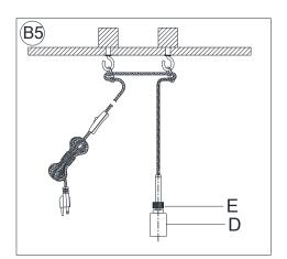
5. Unscrew the Knurled Nut (E) on the Socket (D).
