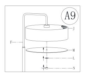
Attach Diffuser (M) and Flat Washer (L) onto center nipple. Screw Final Nut (N) onto center nipple and turn clockwise to tighten securely. Insert the plug into a proper electrical outlet and then turn on the switch.
