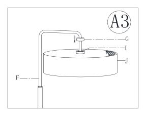
3. Adjust Cover (G) onto Connection Head (I).
