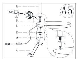
5. Unscrew the Bottom Nut (A) and Washer (B) using the Spanner (O), do not discard the parts as these will be used later. Pull out the Plastic Tube (P) from the hole on the Base (D) then throw it into trash (same as image remark). Put Base (D) onto Lower Tube (E). Make sure Lamp Shade is ahead to front of Base. Screw Bottom Washer (B) and Bottom Nut (A) onto Lower Tube (E). And turn clockwise to tighten securely by the Spanner(O).
