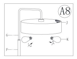
8. Insert the specified light Bulbs (K) into Sockets. DO NOT EXCEED THE SPECIFIED WATTAGE.
