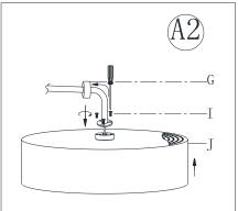
2. Raise the Cover (G) without scratch tube. Put Lamp Shade (J) onto Connection Head (I) aligning with the 3 holes. Fix Lamp Shade (J) by using 3 Assembly Screws (H) and tighten with a screwdriver.
