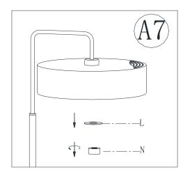
7. Remove Flat Washer (L) and Final Nut (N) from nipple. Do not discard the parts as these will be used later.
