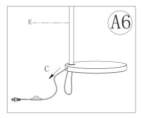
6. Pull Cable(C) out from base and making sure cable is no twist.
