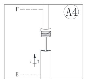
4 . Screw Lower Tube (E) onto Upper Tube (F). And turn clockwise to tighten securely.
