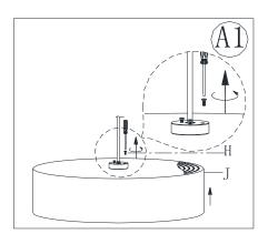
Remove 3 Assembly Screws (H) from top head of Lamp Shade (J).
