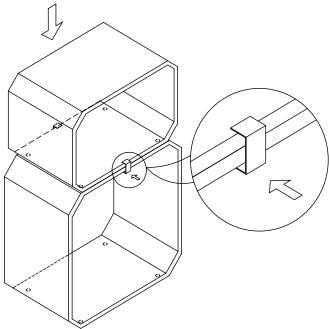
2. Align small size unit onto top of middle unit. Slide bracket (B) over the edge of the two units like the drawing shows.
