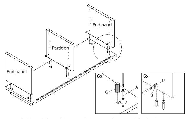
2. Insert 6 dowels (C) into holes in the bottom of the top panel. Using a phillips head screwdriver screw the cam bolts (A) into the bottom of the top panel. Insert cam locks (B) into the end panels and the partition like the drawing shows. Assemble the top panel down onto the end panels and partition aligning the dowels and cam bolts. Tighten cam locks (B) with a phillips head screwdriver.
