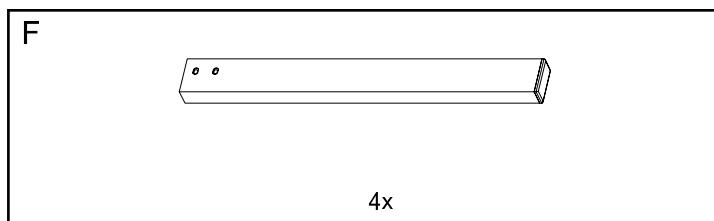
1. Lay the dining table top (E) upside down onto a clean smooth surface such as carpet or cardboard. Align legs (F) as shown. Insert bolt (A), lock washer (B), and flat washer (C). Tighten with supplied hex key (D). Stand table upright.
