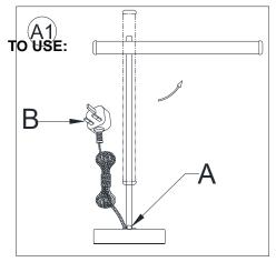
1. Gently rotate the light rod to horizontal position as shown. Insert the Plug (B) into a proper socket. Rotate the Switch (A) to turn on and adjust the brightness of the light.
