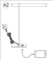
There is one USB Port on the fixture base, which can be used for charging USB devices (USB charging cable is not included). The output maximum is 5V/2A. Do not overcharge.
