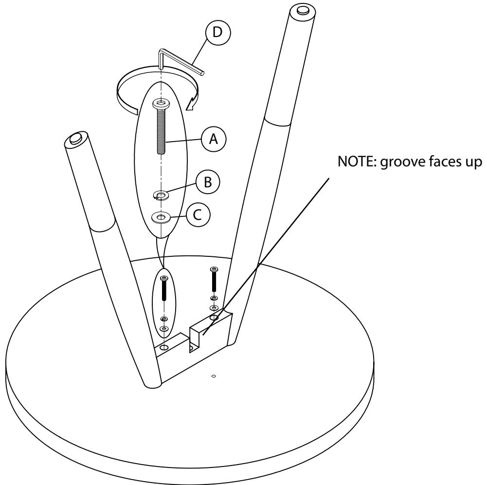
2. Align leg frame as shown in drawing. Insert bolt (A), lock washer (B), and flat washer (C). Tighten with hex key (D).
