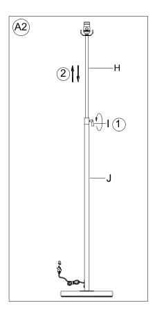
To adjust the Adjustable Tube (H) up and down, turn and loosen the Adjustment Lever (I) by rotating it in a counterclockwise direction, until the desired position is selected
