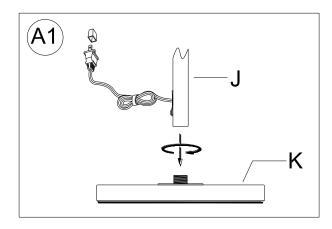
Attach the Bottom Tube (J) onto the Lamp Base (K) by rotating the Bottom Tube (J) clockwise until tight.
