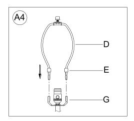
Raise the Harp Caps (E) and insert the bottom ends of Harp (D) into the Saddle (G)  $\,$
