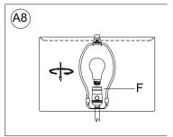
Insert the specified light bulb into the Socket (F). DO NOT EXCEED THE SPECIFIED WATTAGE.
