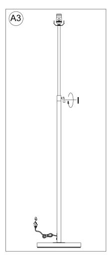
Turning and tighten the Adjustment Lever (I) by rotating it in a clockwise direction until tight.
