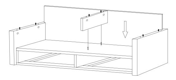
4. Screw cam bolts (F) into top panel. Insert cam locks (E) into holes in side panels, making sure the arrow on the cam locks points towards the hole in the edge of the panel. Set top panel onto side panel, fitting cam bolt into cam locks. Tighten cam locks with a phillips screwdriver.
