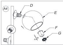
Attach the Glass Shades (E) onto the Sockets (D). Place the Spacers (F) onto the Sockets (D) and then secure Glass Shades (E) and Spacers (F) by rotating the Socket Rings (G) in a clockwise direction until tight.
