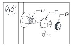
3. Unscrew the Socket Ring (G) and Spacer (F) from each Socket (D) by rotating the Socket Rings (G) in a counter-clockwise direction.
