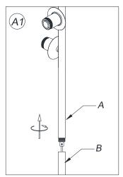
1. Attach the Lower Tube (B) onto the Upper Tube (A) by rotating the Lower Tube (B) in a clockwise direction until tight.
