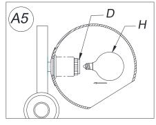
5. Insert the specified light bulbs into the Sockets (D). DO NOT EXCEED THE SPECIFIED WATTAGE.
