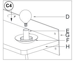
Insert the specified light bulb into the Socket (E). DO NOT EXCEED THE SPECIFIED WATTAGE.
