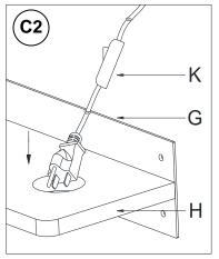
Insert the Plug and Switch (K) through the hole of Wood Shelf (H), and then insert the Knurled Nut (J) & Flat Plate(I) through the hole in order.
