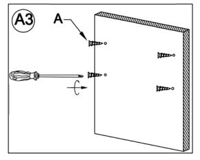
Use a Phillips Screwdriver to insert the Wall Anchors (A) at the marked locations. Do not "push" or pound the Wall Anchors (A) into the wall, it is designed to bore into the wall like a drill bit. Slowly turn the Wall Anchors (A) in a clockwise while applying pressure until the flange of the anchor just touches the wall.
