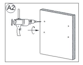
Pre-drill pilot holes at the marker locations. This will make installing the Wall Anchors (A) into the wall easier.
