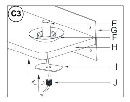
Sit Lamp Cup (F) on the Shelf, rise Flat Plate (I) onto the bottom of the shelf and screw Fixed Nut (J) onto the threaded tube under the Lamp Cup (F).
