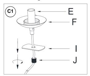
Separate the Flat Plate (I) from the Lamp Cup (F) by unscrewing the Knurled Nut (J).
