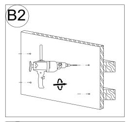
Pre-drill pilot holes at the marker locations. This will make installing the Wall Screws (B) into the wall easier.
