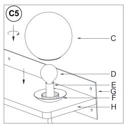
Screw Glass Shade (C) onto Lamp Cup (F). Insert the plug into a proper electrical outlet and turn on the switch to test the fixture.
