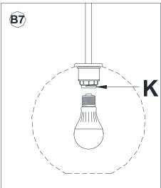
Put the Glass Shades (L) (Packed separately) and Spacers (M) onto the Sockets (K), secure Glass Shades (L) (Packed separately) and Spacers (M) by rotating the Socket Rings(N) in a clockwise direction until tight.
