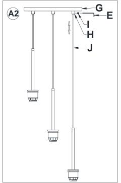
2. Loosen the Set Screws (I) from the Collars (H) under the Canopy (G) using a Allen Wrench (E) by turning counter-clockwise. Adjust the Power Cord (J) upwards or downwards through the Canopy (G) until a new desired suspension length is determined. Secure the Power Cord (J) in place by tightening the Set Screws (I) onto the Collars (H). Do not over tighten the screw, making sure the Power Cord (J) will not slip downwards with the pendant body.
