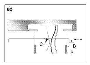
2 Gently pull existing wire down from the ceiling junction box and allow wires to hang. Attach Mounting Plate (F) to the ceiling outlet box, aligning the slots of the Mounting Plate (F) with the two threaded holes located on the J-Box. Insert and tighten 2 Mounting Screws (B) with a screwdriver.
