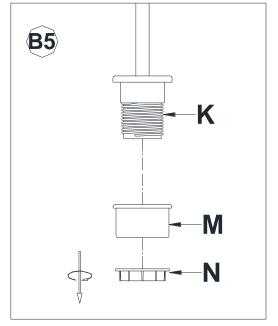
5. Unscrew the Socket Rings (N) and Spacers (M) from the Sockets (K).
