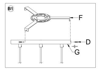
1. Separate the Mounting Plate (F) from the Canopy (G) by removing the 3 Canopy Screws (D). Do not discard the Canopy Screws (D) as these will be used later.
