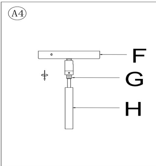
4. First thread the fixture's 3 wire power cord through the Swivel (G) and Canopy (F) and then attach the Swivel (G) onto the assembled Metal Tubes (H/J) by rotating the 2 parts clockwise until tight.
