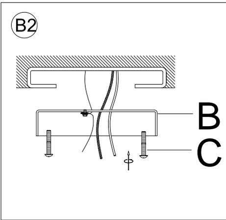
2. Gently pull existing wire down from the ceiling junction box and allow wires to hang. Attach Mounting Plate (B) to the ceiling outlet box, aligning the slots of the Mounting Plate (B) with the two threaded holes located on the J-Box. Insert and tighten 2 Mounting Screws (C) with a screwdriver.
