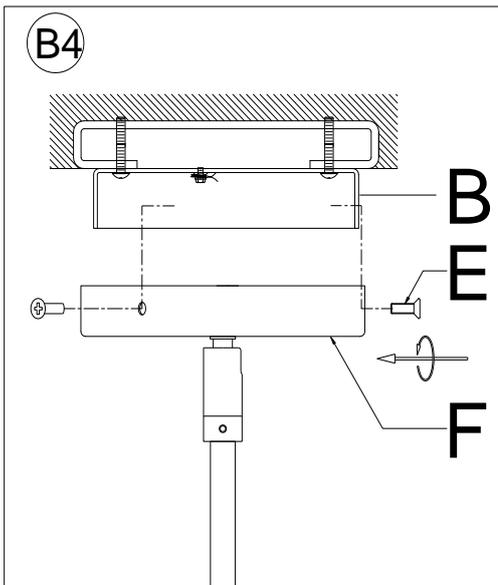
4. Raise Canopy (F) up over the Mounting Plate (B), align the 3 holes on the Mounting Plate (B) with the 3 holes on the side of the Canopy (F). Insert 3 Canopy Screws (E) and tighten to secure the Canopy (F) with a screwdriver.
