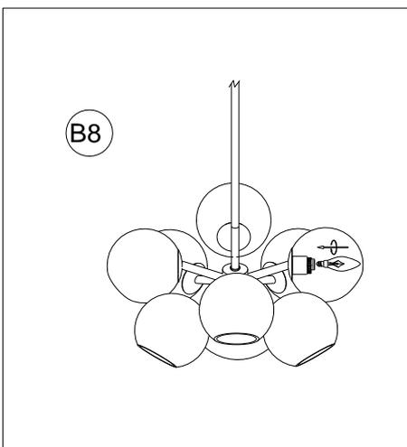
8. Insert the specified light bulbs into the Sockets (K) and Socket (Q). DO NOT EXCEED THE SPECIFIED WATTAGE.
