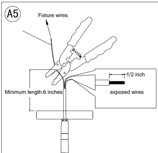
5. If needed, cut off the extra power cord length on the 3 wire cords so that they all are at least 6 inches (152.4 mm) long within the outlet junction box (J-box).
