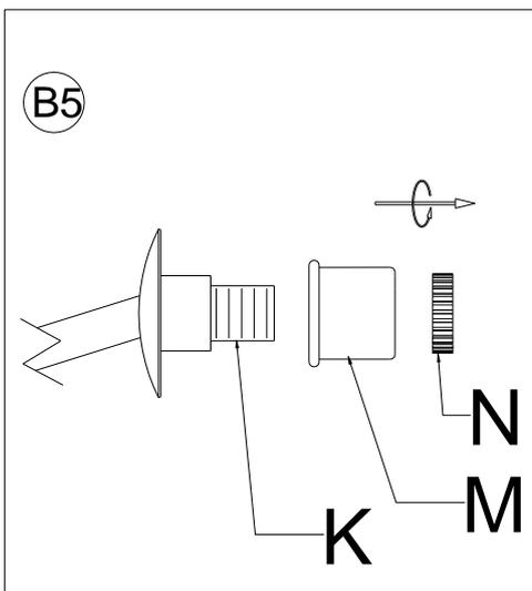
5. Unscrew the Socket Rings(N) and Spacers (M) from the Sockets (K) and Socket (Q) by rotating the Socket Rings (N) in a counter-clockwise direction.
