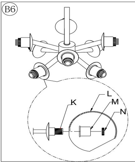
6. Attach the 8 Glass Shades A (L) onto the Sockets (K). Place the Spacers (M) onto the Sockets (K), Secure Glass Shades A (L) and Spacers (M) by rotating the Socket Rings(N) in a clockwise direction until tight.
