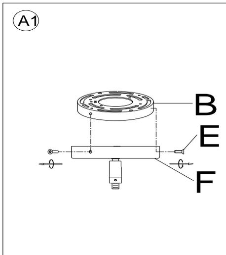
1. Separate the Mounting Plate (B) from the Canopy (F) by removing the 3 Canopy Screws (E). Do not discard the Canopy Screws (E) as these will be used later.
