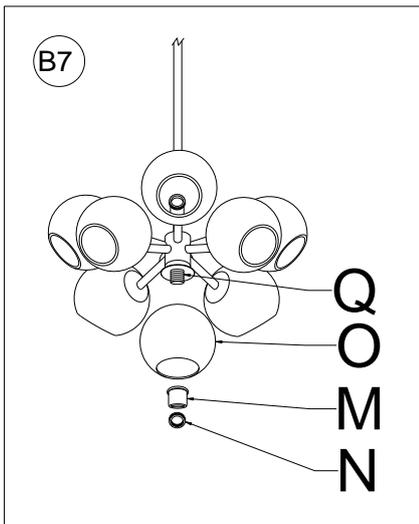
7. Attach the Glass Shade B (O) onto the Socket (Q) at the bottom of fixture. Place the Spacer (M) onto the Socket (Q), Secure Glass Shade B (O) and Spacer (M) by rotating the Socket Ring (N) in a clockwise direction until tight.
