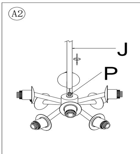
2. Insert the fixture 3 wire power cord through the 6 in. Tube (J), and attach bottom end of the 6 in. Tube (J) onto the Threaded Pipe (P) by turning clockwise until tight.
