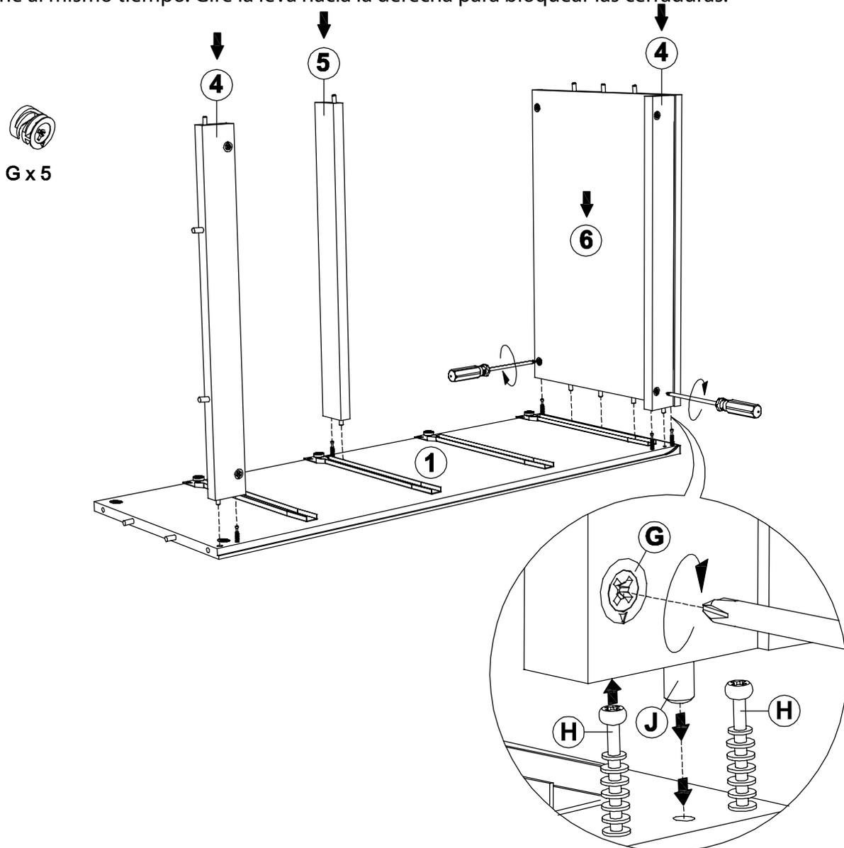
9. Insert large cam locks (G) into rails and panels as shown. Align right side panel and press together make sure the dowels line up. Turn Cam locks clockwise to lock.
