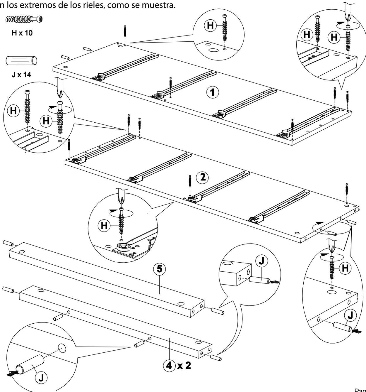
7. Insert large cam bolts (H) into top panel. Insert large dowels (J) into bottom panel as shown below. Align back rail and press together with bottom panel.
