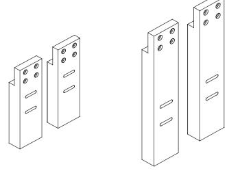
2. Fasten legs to the headboard using bolt (E), lock washer (B), flat washer (C), and cap nuts (F), in order as shown. Tighten with supplied allen key.
