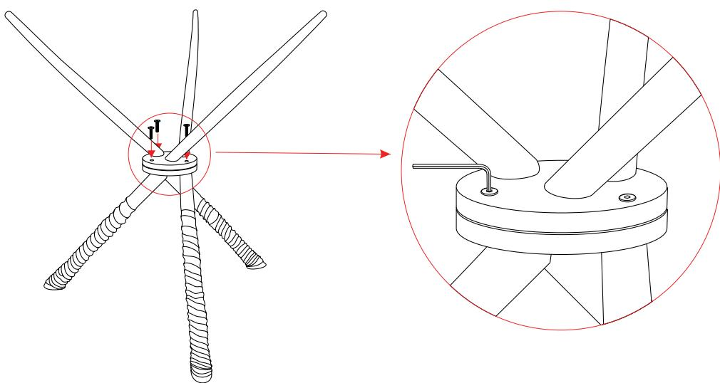
3. Flip table base over. Insert pads (C) as shown. Align glass top as shown.
