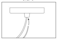
7. Insert the steel cable into the cable stop and tighten the cable screws with a small screwdriver.
