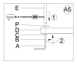
5. Attach the Lower Tube (E) onto the Lamp Base (D). Insert the Large Allen Screw (B) with Metal Washer (C) into the bottom threaded hole of the Lamp Base (D) and Lower Tube (E).
