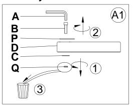
Loosen the Hex Nut (Q) from Lamp Base (D) using Large Allen Key (A). Discard the Hex Nut (Q).
