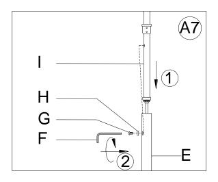
7. Insert the Upper Curved Tube (I) into the Lower Tube (E), and aligning the screw hole on Upper Curved Tube (I) with the hole on the Lower Tube (E). Secure Medium Allen Screw (G) and Round Nut (H) onto the Lower Tube (E) using the Medium Allen Key (F) until tight.
