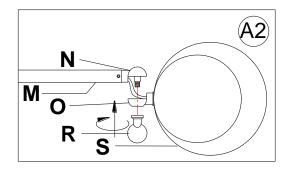
2. Insert the Metal swivel on right (N) into the Metal swivel on left (O) and Secure the Metal swivel on left (O) onto Metal swivel on right (N) by turning the Knob (R) in a clockwise
