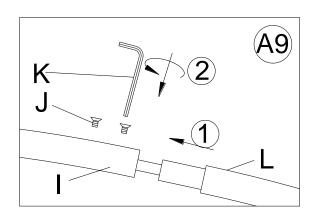
9. Insert the Middle Curved Tube (L)into the Upper Curved Tube (I)., aligning the screw holes on Middle Curved Tube (L) with the holes on the Upper Curved Tube (I). Secure the Set Screws (J) into the holes on the Upper Curved Tube (I). using Small Allen Key (K) until tight.
