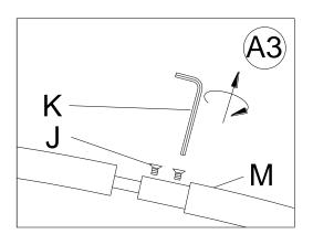
3. Loosen the Set Screws (J) from Top Curved Tube (M) using Small Allen Key (K).
