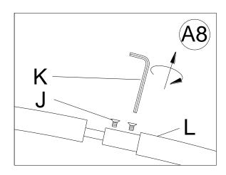
8. Loosen the Set Screws (J) from the Middle Curved Tube (L) using the Small Allen Key (K).
