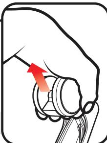
**03** Insert your static stands by fully pressing in each stem into the respective wheelbase sockets.
