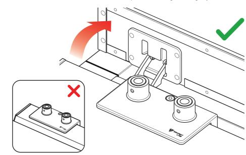
Tighten the set screws on both the upper arms and the clamp mount to lock the arms in place.
