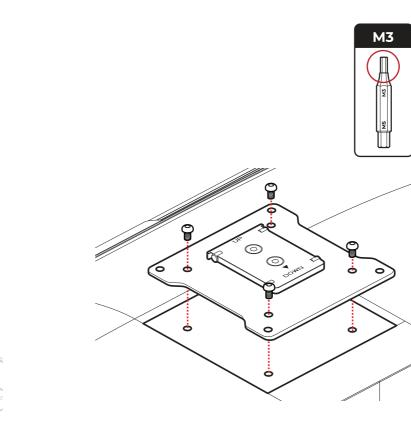
**103** Fully tighten the top screw **clockwise** to anchor the clamp in place.
