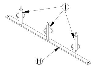
7. Attach this assembled Supporting Rail (H) and Support Leg (I) with Slats Roll (G). Connect the 1<sup>st</sup> slat to the end of Supporting Rail (H). This can be done by inserting Hex Bolt (L) followed with spring washer (M) and flat washer(N) through the pre-drilled hole in 1<sup>st</sup> slat, and into the pre-drilled holes in Supporting Rail (H). Tighten with Allen Key (K). Repeat at the other end.
