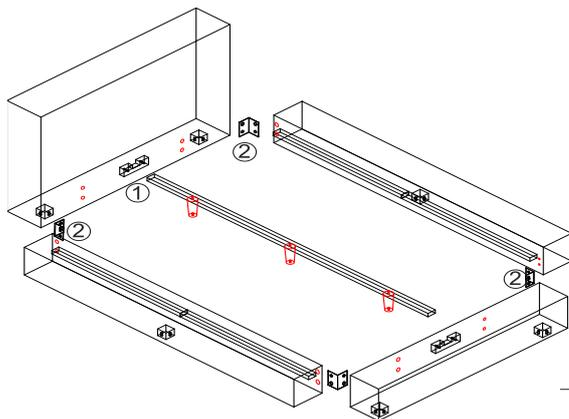
① Attached the Wooden Leg (F) to the side rail, Footboard and HeadBoard, insert the Screw(E) and tighten with Philips head screwdriver.
