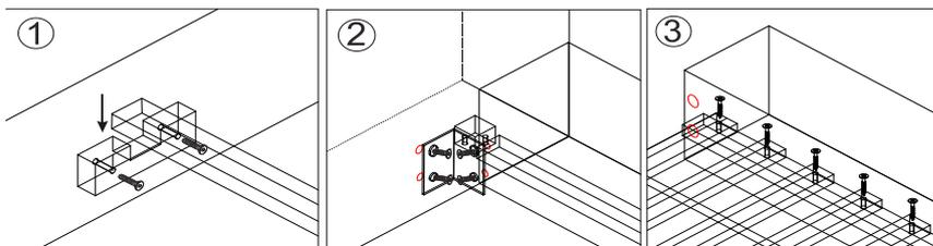
③ Lay the wooden slat roll in between the Headboard and the Footboard, secure the Wooden Slat Roll to the bed frame using screw (D), tighten with the Phillips Head Screwdriver (not included). Tighten up all bolts and screws to make sure the bed structure is rigid. It is recommended all screws be checked from time to time for safety as the hardware may loosen over time.
