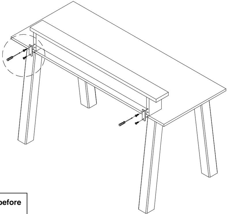
**Make sure the holes are aligned before tighten the screws.**
