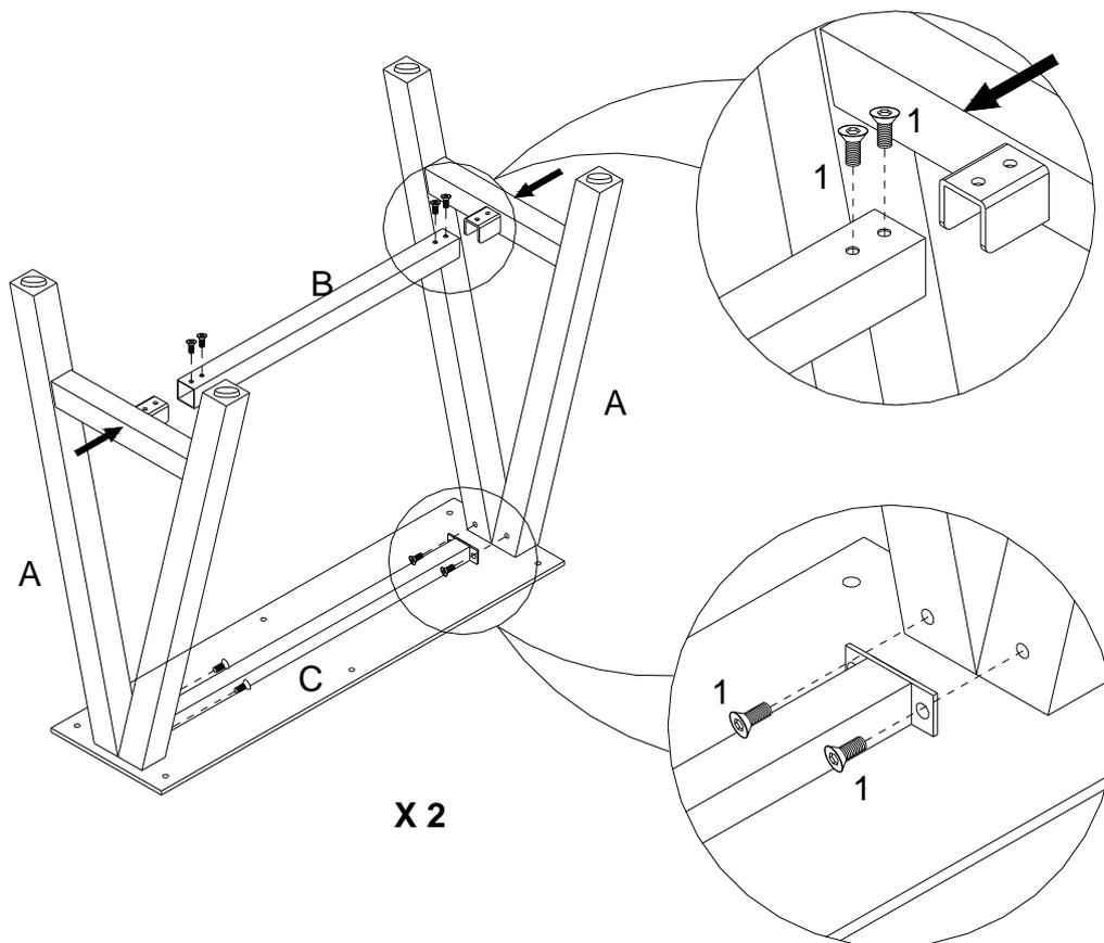
2. Secure the Metal Plate(C) to A Frames(A) using bolts(1) , tighten by hand at first, securely tighten the bolts with Allen wrench(5), but do not over tighten the bolts.
