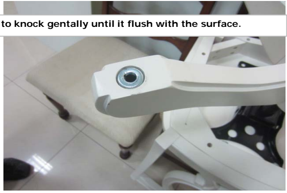
use hand force or rubber mallet to force the cartor pin into the bushing
