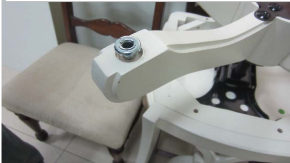
replace the socket on the hole, use metal hammer to knock gently until it flush with the surface.
