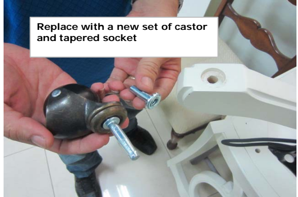
replace the socket on the hole, use metal hammer to knock gently until it flush with the surface.
