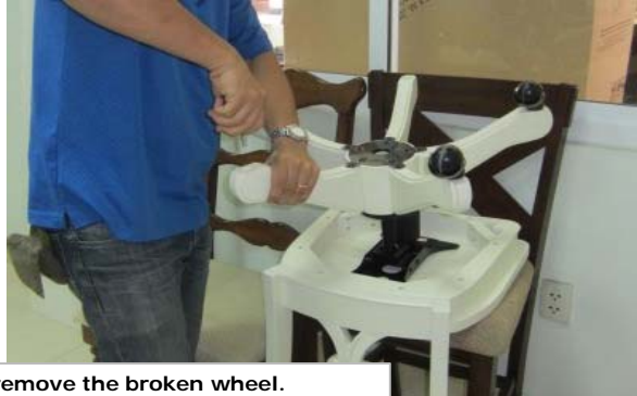
Pull out or use rubber mallet to remove the broken wheel.
