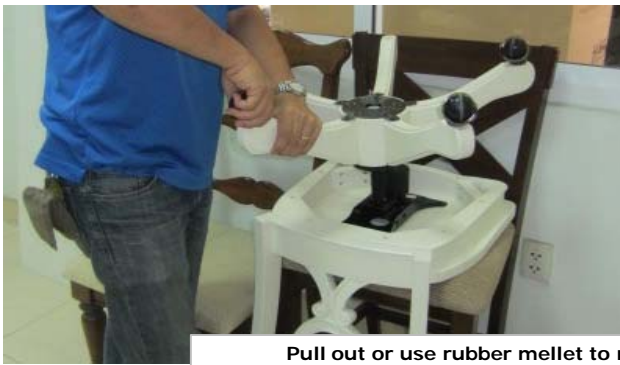
Pull out or use rubber mallet to remove the broken wheel.
