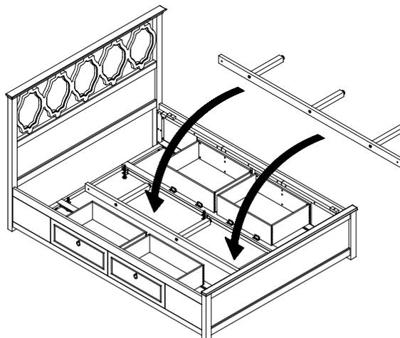
11. Lay the Slats (E) halfway on top as shown below. Tilt up the Slats Support Strether (G) afix with the Slats Support Legs (H) in a standing position as shown below.
