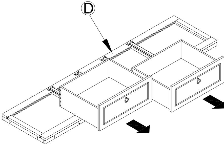
2. Attach the Drawer Boxes (D) bottom panels to the Siderails (C) as shown below. Place the Flat Washer (Q), Spring Washer (P) and followed by the Short Allen Bolt (O) – 3sets; into the pre-drilled holes of the Drawer Boxes (D) bottom panel into the Siderails (C) and tightening using the Ball Tip Allen Key (J) as shown below.
