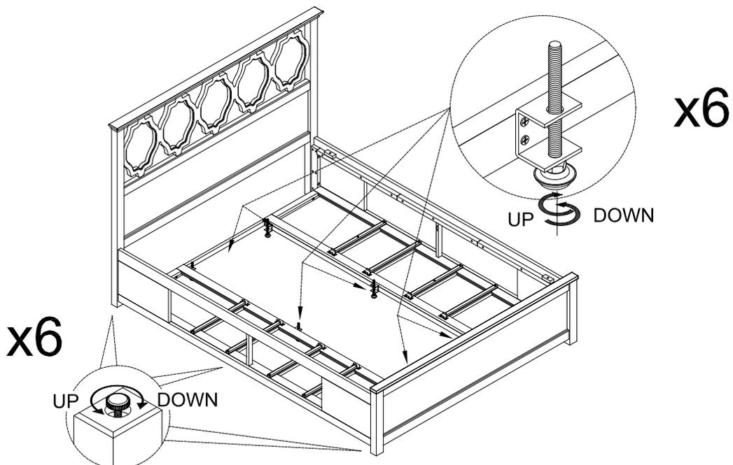
8. Insert the Drawer Boxes into the original places as Drawer Boxes with Frame (D) as shown below.
