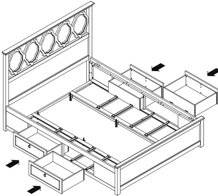
9. Attached the Slats Support Legs (H) into the pre-drilled holes of the Slats Support Stretcher (G) by turning the Slats Support Legs (H) in a clockwise direction for tightening as shown below.
