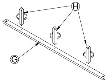
10. Place the Slats Support Stretcher (G) affix with the Slats Support Legs (H) onto the surface floor in between the Bed as shown below.
