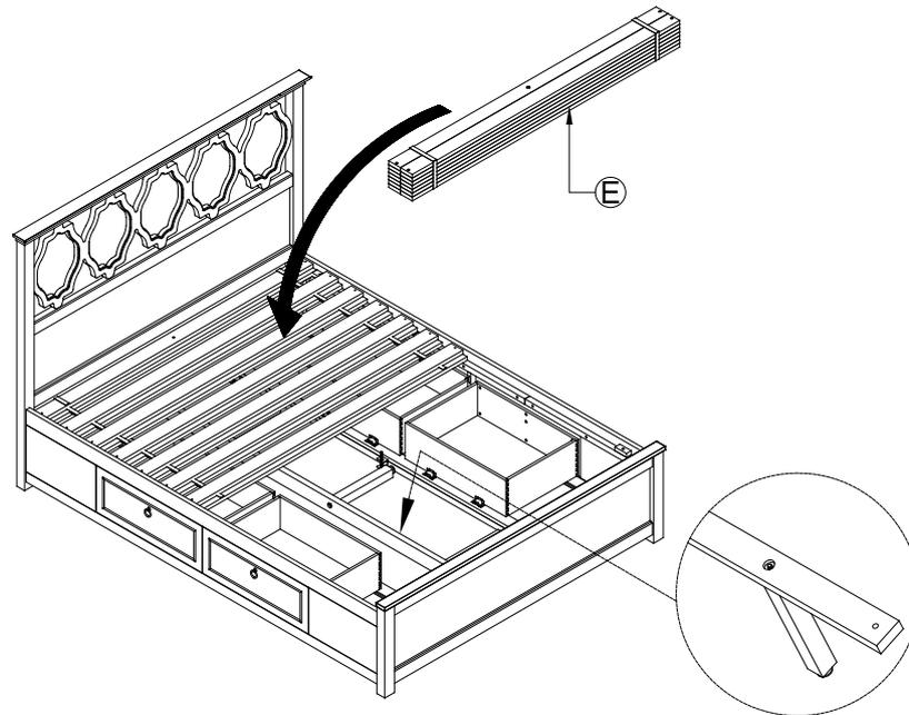
12. Attached the Slats Support Strether (G) afix with the Slats Support Legs (H) to the pre-drilled holes of the Slats (E) by placing the Flat Washer (Q), Spring Washer (P) and followed by Medium Allen Bolt (N) on the center surface of the pre-drilled holes of Slats (E). Tighen it by using the Ball Tip Allen Key (J). After fixing on the 1<sup>st</sup> Medium Allen Bolt (N), fully extend the Slats (E). Illustration as shown below.
