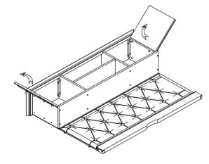
4. Attach the upper case (A), pin board (B) to the Side Panel (C&D). insert 4pcs wooden dowel into the pre-drilled holes on the upper case (A) and side panel (C) and (D). Insert 8 set of bolt 2 (e), Spring Washer (b), Flat Washer (c) and tighten the bolt with Allen key (h)
