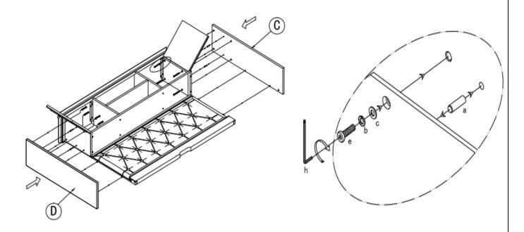
5. Insert 2 sets of Bolt 1 (d), Spring Washer (b), and Flat Washer (c)) into the holes at the back rail of the pin board (B) and side panel (D&C) and tighten the bolt with Allen key (h), as show below
