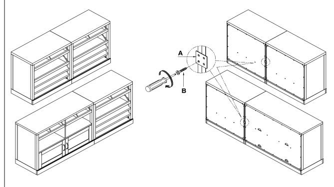
**6.** NOTE: Installation of the Anti Tip Kit is REQUIRED. Please follow the separate instructions to secure the Art consoles to the wall, by using the tipping-restraint kit included.
