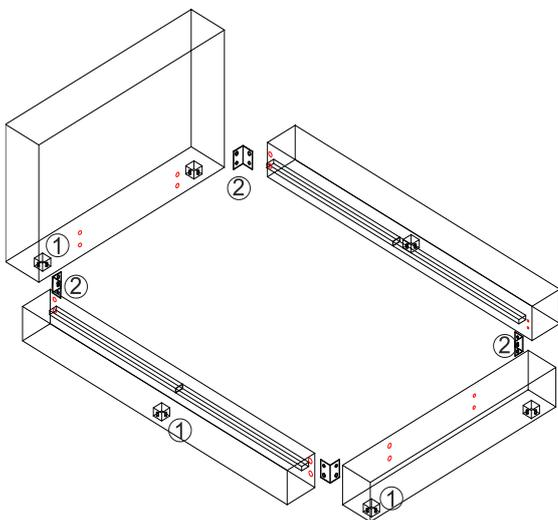
① Attached the Wooden Leg (E) to the side rail, Footboard and HeadBoard, insert the Screw (D) and tighten with Phillips head screw driver.
