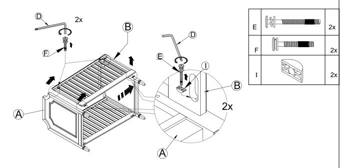
3. Attach (N) to (A) by aligning pre-drill holes with wooden dowels as shown below. Do not fully tighten bolts (E & F) at this point to make installation of the Mattress Base (C) easier.
