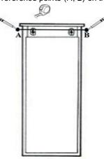
Connect the two points (A, B) with a light pencil line. Use a level to ensure that the line is level.
