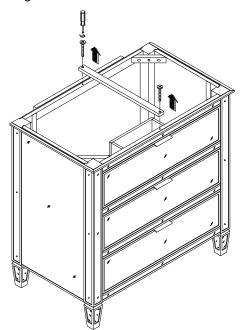
5. Before placing the Console Top Frame on top the Console Top (A), please remove the Screws (2pcs) from the Center Stability Support Rail and remove the Support Rail away as well. As seen in the illustration above.
