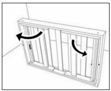
3. Once legs are pulled out of the tray stand, ensure to securely lock the latch on the center of the upper legs of the base/stand to make it firm.
