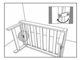
4. After locking the latch, put the stand on its functional position.
