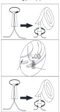
9. Connect the NEUTRAL FIXTURE WIRE to the NEUTRAL JUNCTION BOX WIRE (usually white insulation). Fasten each together with a Plastic Wire Nut Connector (H) by twisting the connector in a clockwise direction and wrap the connection with electrical tape. Be sure that no wire strands are exposed.
