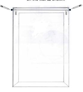
3 Connect the two points (A, B) with a light pencil line. Use a level to ensure that the line is level.
