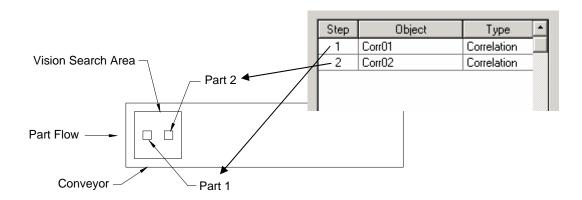
If the vision sequence used to locate the parts is more complex, then the last two objects of the sequence must have the location for parts 1 and 2. The object that finds part 1 must be the second to last object. The object that finds part 2 must be the last object. For example, the following sequence uses two Point objects for the locations of part 1 and part 2. Step 5 locates part 1 and step 6 locates part 2.
