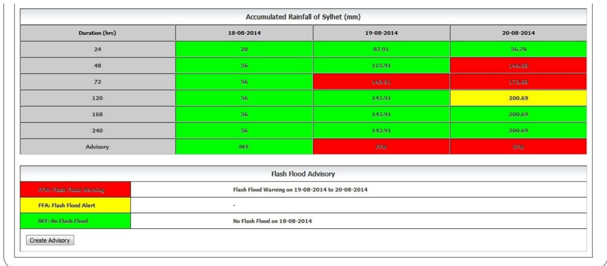
Figure 6.3 : Module for analysis of flash flood potential (red for flash flood warning; yellow for alert; green for no flood threat)
